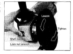
To remove the disc, follow the installation procedure in reverse.
